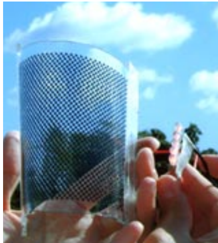
A new spherical solar cell module which is flexible and can utilize light in all directions
